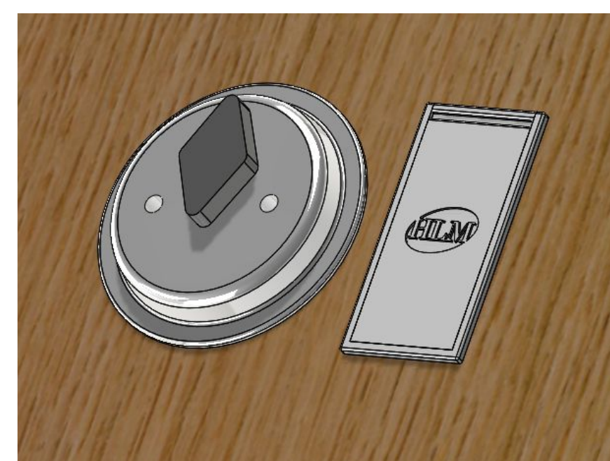
Fig. 4: invasive sensor installation mock up
